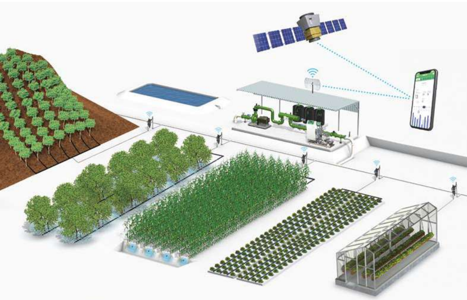
Schematic layout of various drip irrigation systems with interfaces for smart technology
